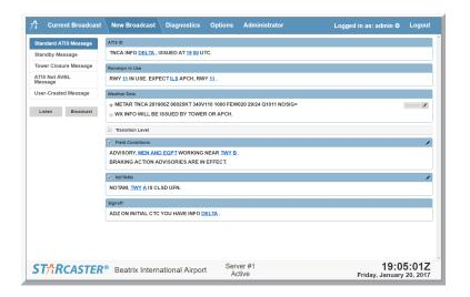
**STARCASTER®** is a **Natural Voice Text-to-Speech** system that provides the controller with a way to easily create clear and consistent broadcasts.
