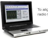
To align and maintain a Fylde SuperTrunk III system, you just need a standard radio test set and a laptop PC running the Fylde Field Programmer software.
